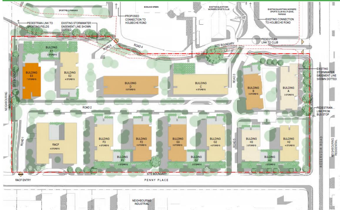
Figure 11: Proposed Block layout and building storeys (Source: Architectural Plans).
